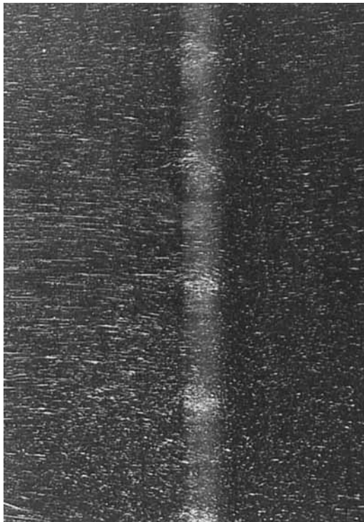
FIGURE 21. Plane view of flow in a plane perpendicular to the flow in regime D: A1 method, d = 1.0 cm, a = 1.0 cm, f = 0.206 Hz, KC = 6.28 , \beta = 22.4 , t_e = 60 s.
