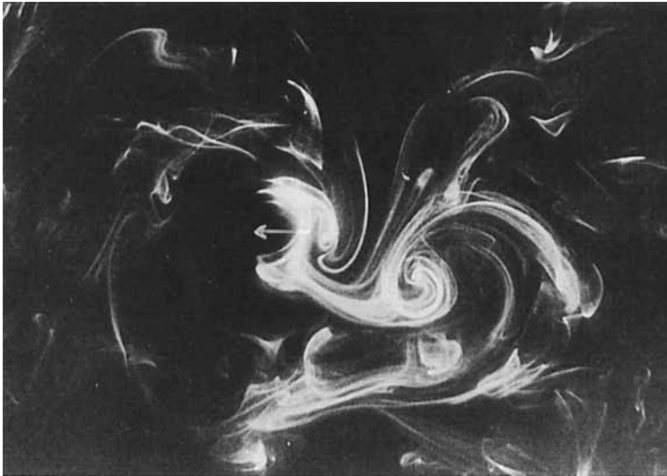
FIGURE 32. Plane view of flow in the (X, Y) -plane in regime G: e.p. method, d = 2.0 cm, a = 2.63 cm, f = 0.10 Hz, KC = 8.26 , \beta = 37.7 , t_e = \frac{1}{15} s.
